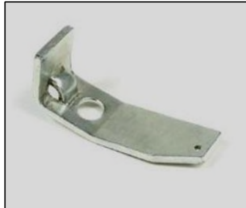
Later '58 and '59 female hood lock lever; long design.
