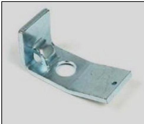
1st design female hood lock lever; short style lever used through approx. 12/11/57.
