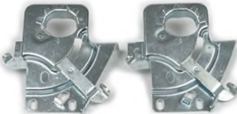
1st design female hood lock lever; short style lever used through approx. 12/11/57.
